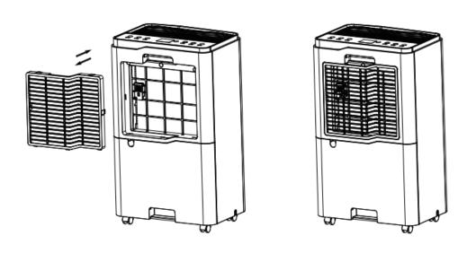
2.Use a vacuum cleaner to gently absorb the dust on the surface. If the filter is very dirty, wash it with water and a soft detergent and dry it thoroughly afterwards.
